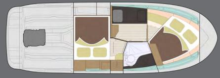
Length: 9,46 M / 31' Beam: 3,22 M/ 11' Draft: 0,97 M/ 3' 2'' Weight (empty boat): 4.5 tonnes Water tank: 280 L/ 73 gallons Blackwater tank: 150 L/ 39 gallons Fuel tank: 440 L/ 116 gallons Batteries: 3+1 (380 AH)
