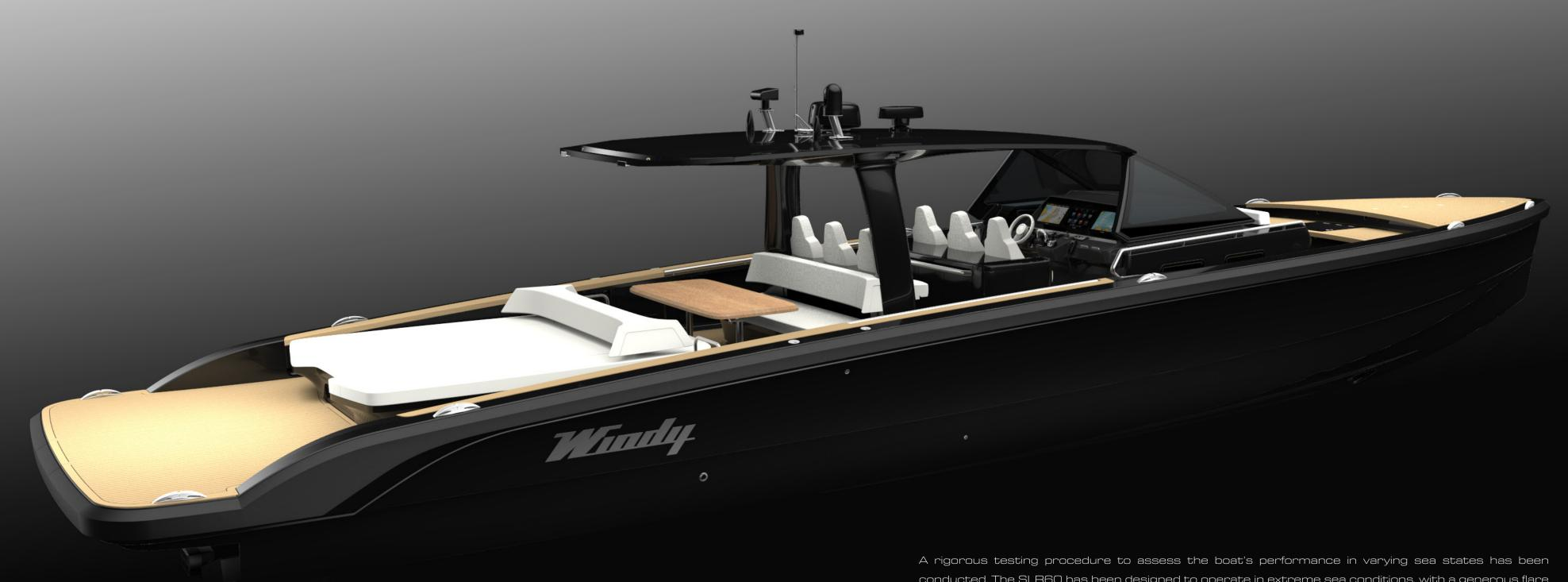
conducted. The SLR60 has been designed to operate in extreme sea conditions, with a generous flare to the bow and multiple chines on the hull keeping the boat as dry as possible.
